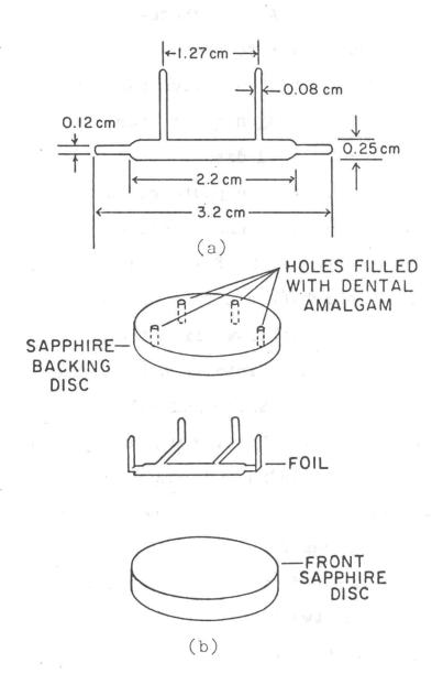
Fig. 2. Details of foil-anvil sandwich.
